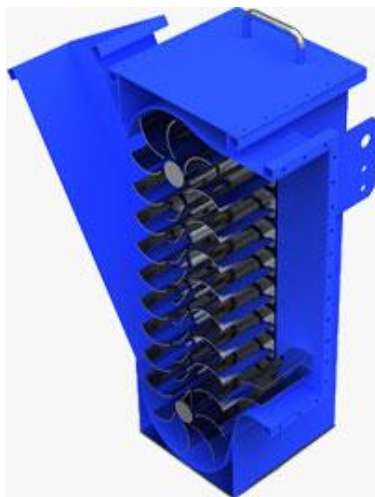
FIGURE 26: CROSS SECTION OF THE HYDROENGINE ( WWW.NATELENERGY.COM )
