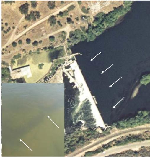
**Figure 8.** Aerial photograph with an inset photograph showing the location and presence of the 1904 log crib dam.
